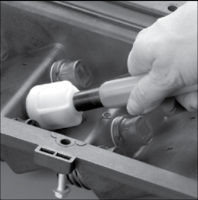
Installation of Hardened Connectors
